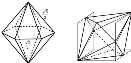
**Fig. 1.** H (Hexagonal bipyramid imaginary cube). This object is projected to a square in six different ways.
